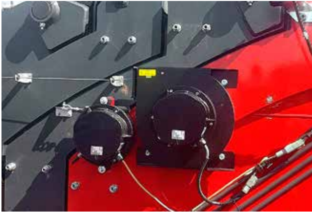
Potentiometer for angle and length of boom detection with redundant safety.
