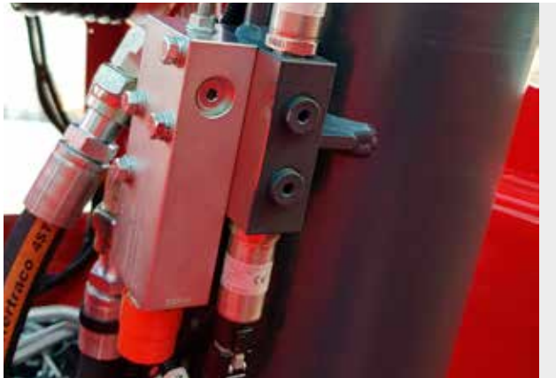
Detection of load weight through 4 pressure transducers: 2 placed on lifting cylinders and 2 on compensation cylinder.
